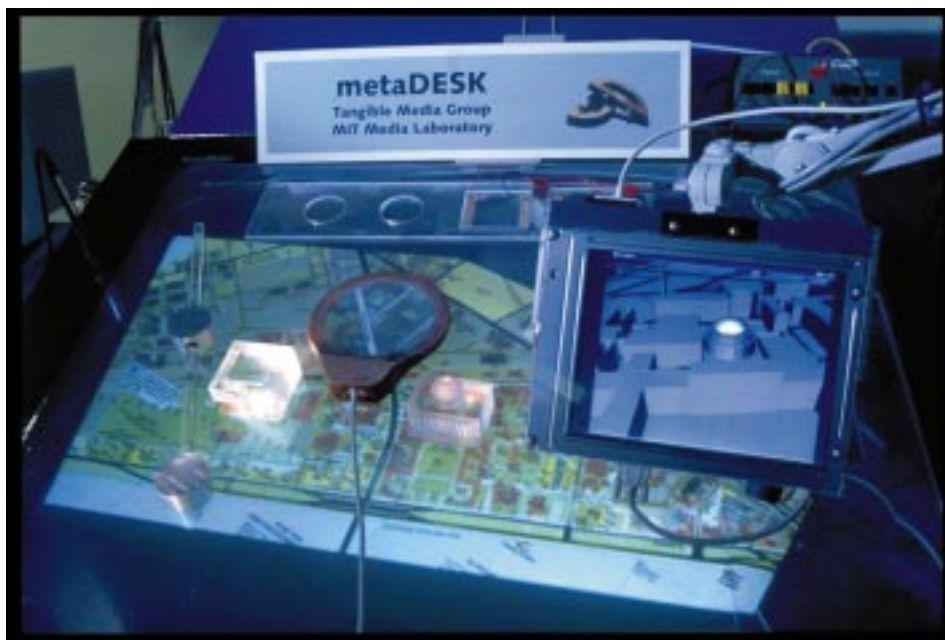
An overview of metaDesk. Real and virtual objects meaningfully coexist in the metaDesk environment. A 2D graphical map is rear-projected onto the desk surface. The placement and orientation of special landmarks (3D physical objects made of plexiglas) are tracked by electronic sensors; changes are reflected in the map beneath. At the right of the picture, a movable “information lens” displays a synthetic 3D rendering of the scene.
