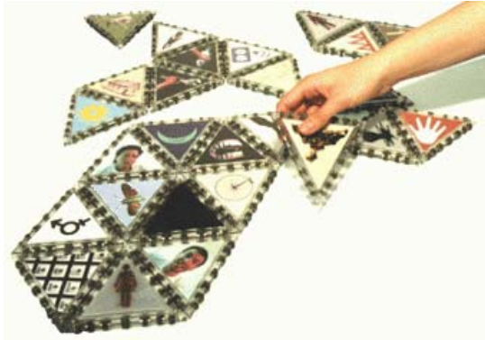
Figure 4: Triangles is a tangible interface in the form of a physical/digital construction kit of plastic triangular pieces.
